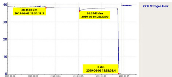
FIG. 2. Labels (left to right) indicate nitrogen flow reduction, due to valve closing, backup system's first stage runs out of nitrogen, and eventually second stage runs out of nitrogen. Zero nitrogen flowed to RICH on 2019-06-06 at 15:33.
